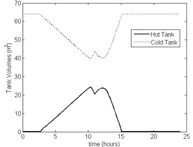
**Figure 6: Storage tank volumes vs time (NMPC).**
