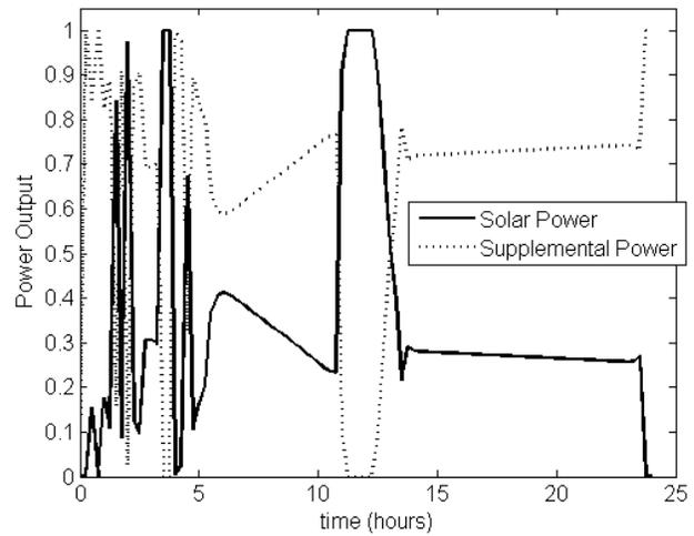
**Figure 8: Solar and supplemental power (dynamic optimization).**
