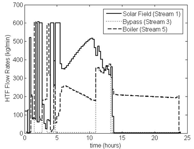
**Figure 9: Mass flow rates (dynamic optimization).**
